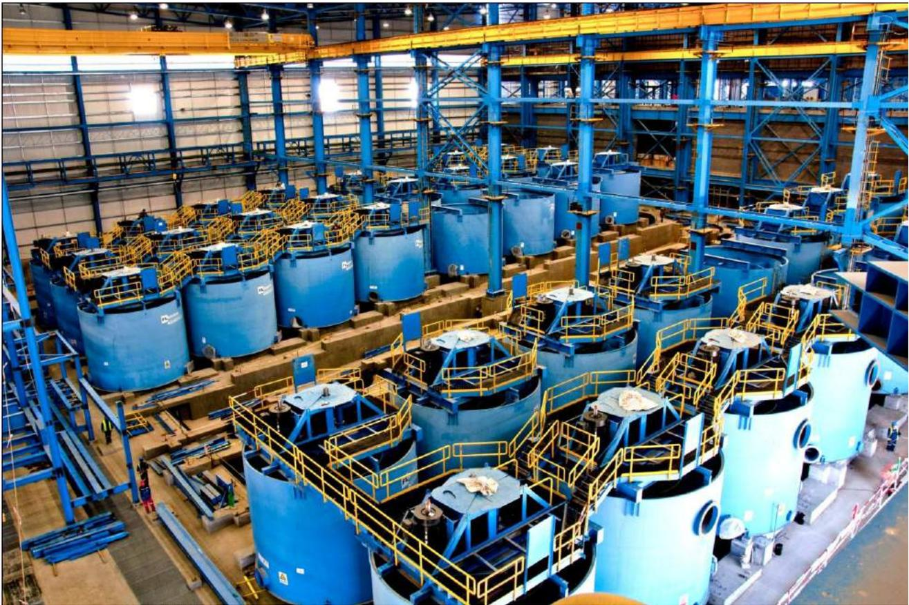
Flotation tanks installed in the concentrator
